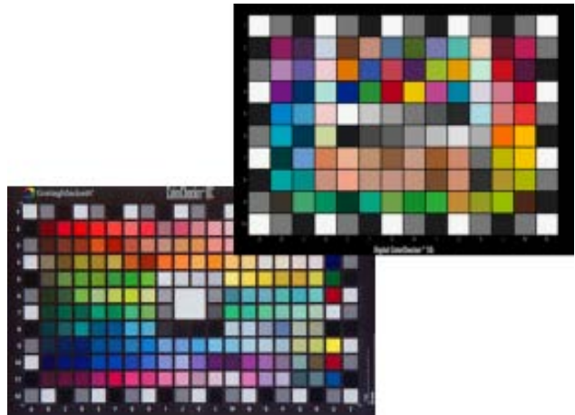
Figure 2. Two generations of the test target X-Rite ColorChecker DC.
