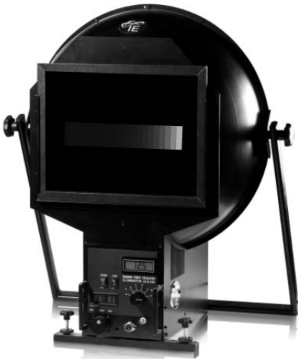
Figure 4. Spherical transparency illuminator.
